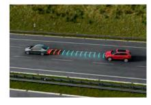
Helping you stay in the intended lane of travel, Lane Assist uses a camera to detect road markings, and supports steering if you veer too close to the edge.
