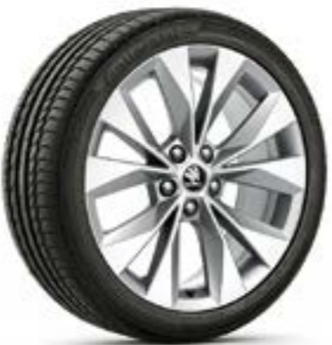
Cassiopeia 3V0 071 498B 8Z8 brushed light-alloy wheel 8.0J x 18" for 235/45 R18 tyres in silver design
