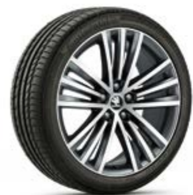
Sirius 3VO 071 499B HA7 brushed light-alloy wheel 8.0J x 19" for 235/40 R19 tyres
