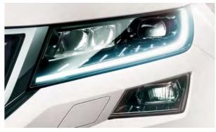
FULL LED HEADLIGHTS WITH ADAPTIVE FRONT LIGHT SYSTEM AND LED DAYTIME RUNNING LIGHTS, LED FRONT FOGS WITH CORNERING FUNCTION
